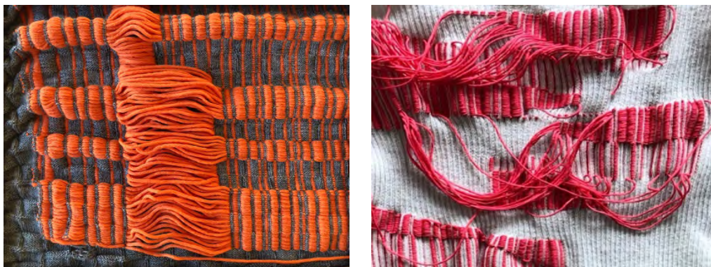
Figures 4 and 5. Pattern subtractions generate long inlay yarn floats
